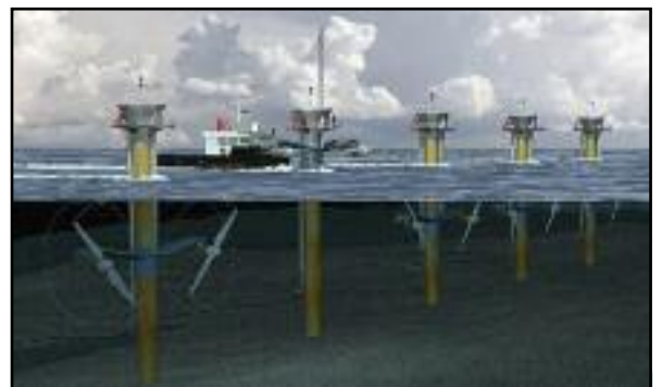
Figure 3.5 SeaGen tidal power generator in Strangford Lough. (www.seageneration.co.uk)
