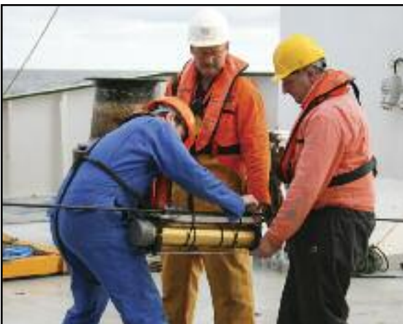
Figure 5.5. IWDG Deep C-POD static acoustic monitoring unit being deployed at 500m in 3000m of water from the RV Celtic Explorer . (© Dave Wall / IWDG).
