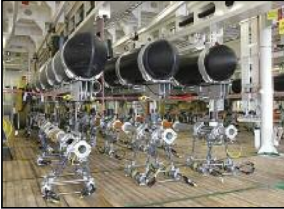
Figure 5.2. Seismic airgun array on deck of ship. (Photo: www.rolls-royce.com).
