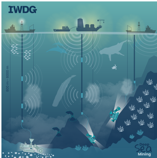
An infographic showing the processes involved in deep sea mining for the three main types of mineral deposit. Schematic not to scale.
